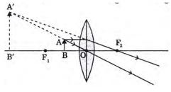
82. One half of a convex lens of focal length 10 cm is covered with a black paper. Can such a lens produce an image of a complete object placed at a distance of 30 cm from the lens? Draw a ray diagram to justify your answer.
