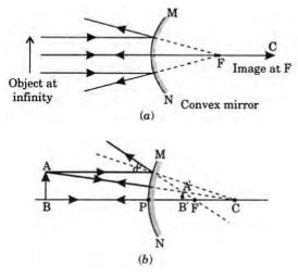
Convex mirrors are used in automobiles as a rear view mirror because of wider field of view and formation of erect image.
