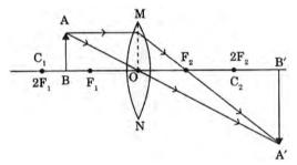
When object is placed in between  $F_1$  and optical centre O of a converging lens, it will form a virtual magnified image of the object.
