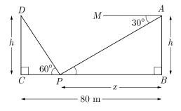
Here distance between pole CD and P is 80 - x. In right angle triangle  $\triangle ABP$ ,  $\angle APB = 30^{\circ}$
