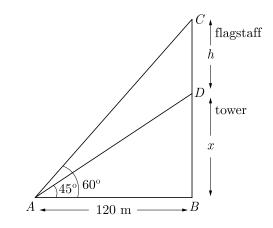
Here  $\angle DAB = 45^{\circ}, \angle CAB = 60^{\circ}$ and AB = 120 m In right angled  $\triangle ABD$  we have
