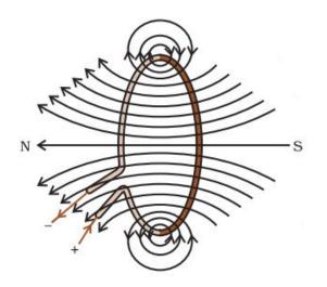
• The magnetic field is represented by concentric circles, with larger circles as one moves away from the loop.
