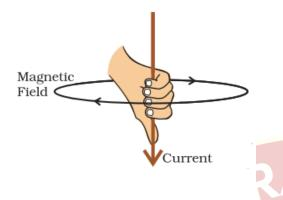
If we imagine that we are holding a currentcarrying straight conductor in our right hand such that the thumb points towards the direction of current. Then our fingers will wrap around the conductor in the direction of the field lines of the magnetic field
