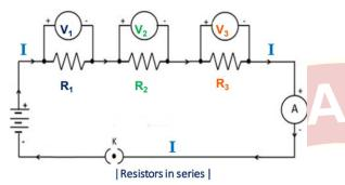
When two or more resistors are connected in series:
